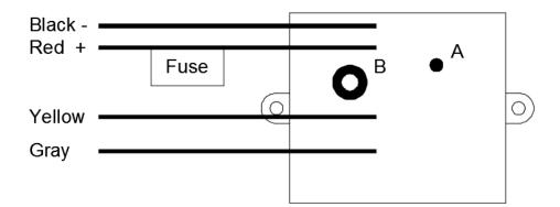
Connect the Black and Red wires to 12 VDC power source (be sure to observe polarity noted). Make sure the amperage capacity of the power source meets or exceeds the requirements of the DC motor being operated with the unit.
