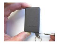
Carefully use a small screwdriver to pry open the case.
