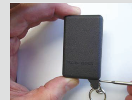
Carefully place small screw driver and pry open case.
