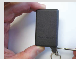
Carefully place small screw driver and pry open case.
