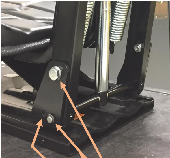
Frame pivot bolt E-ring Rear pivot hole Lower pivot rod Forward pivot hole
